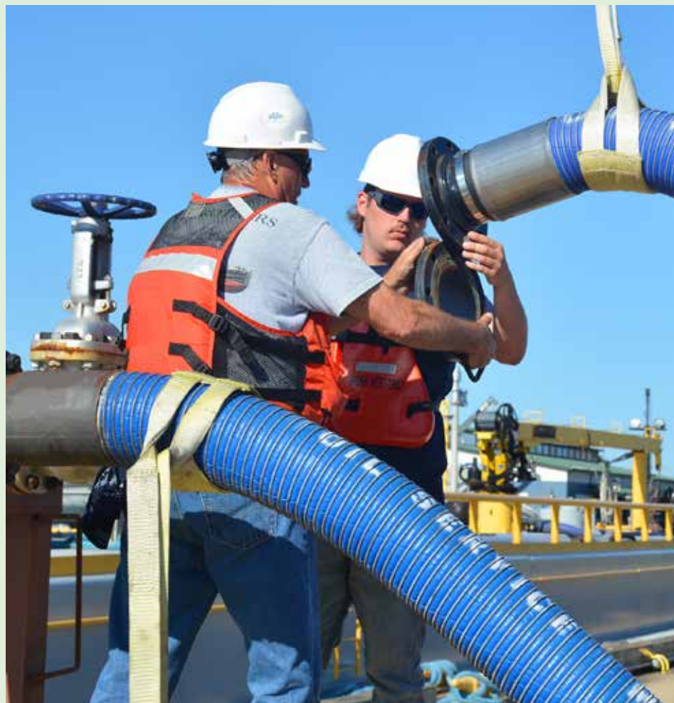
▲ As part of Tankerman Training in June at Vane Brothers' Baltimore headquarters, Vane Marine Superintendent Rich Butrim works with OS Deckhand Nathaniel Tyler, who joined the company in August 2023, on the proper removal of a cargo hose blank prior to connecting to the dock header.
